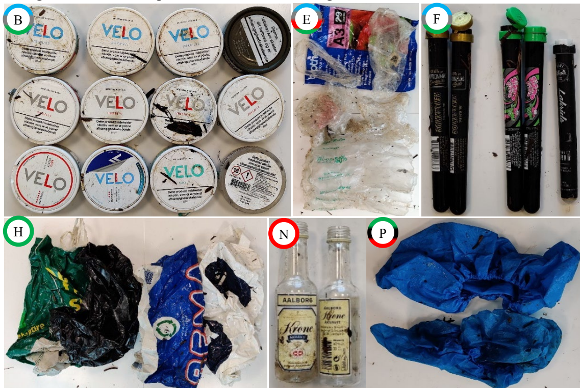
Figure 10: Multi-component litter fractions made of different plastic types are gathered; Blue : PP, Green : PE-LD+PE-LLD, Grey : PE-HD, Red : PET and Black : Rubber.
