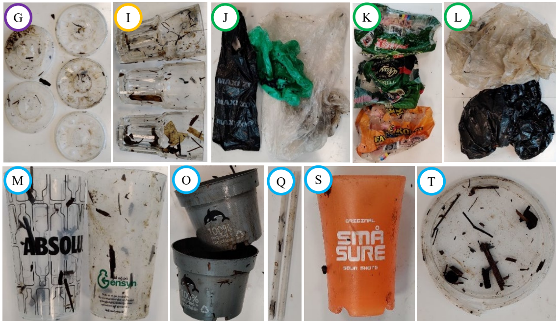
Figure 8: Mono-material litter fractions are gathered; Green with fraction J, K and L: PE-LD+PE-LLD, Orange with fraction I: PC, Blue with fraction M, O, Q, S and T: PP, and Purple with fraction G: PS.
