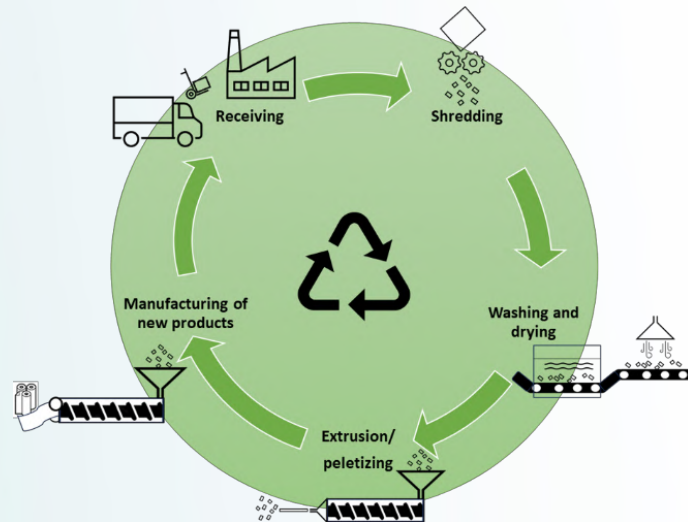
Figure 12 – Simplified schematic diagram of the recycling process [diagram made by PCD]
