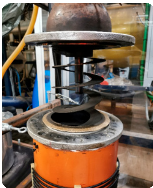
Fig. 5 Internal mixing element of the batch pyrolysis reactor. The screw-shaped mixing element was used to move and mix the plastic material during heating.
