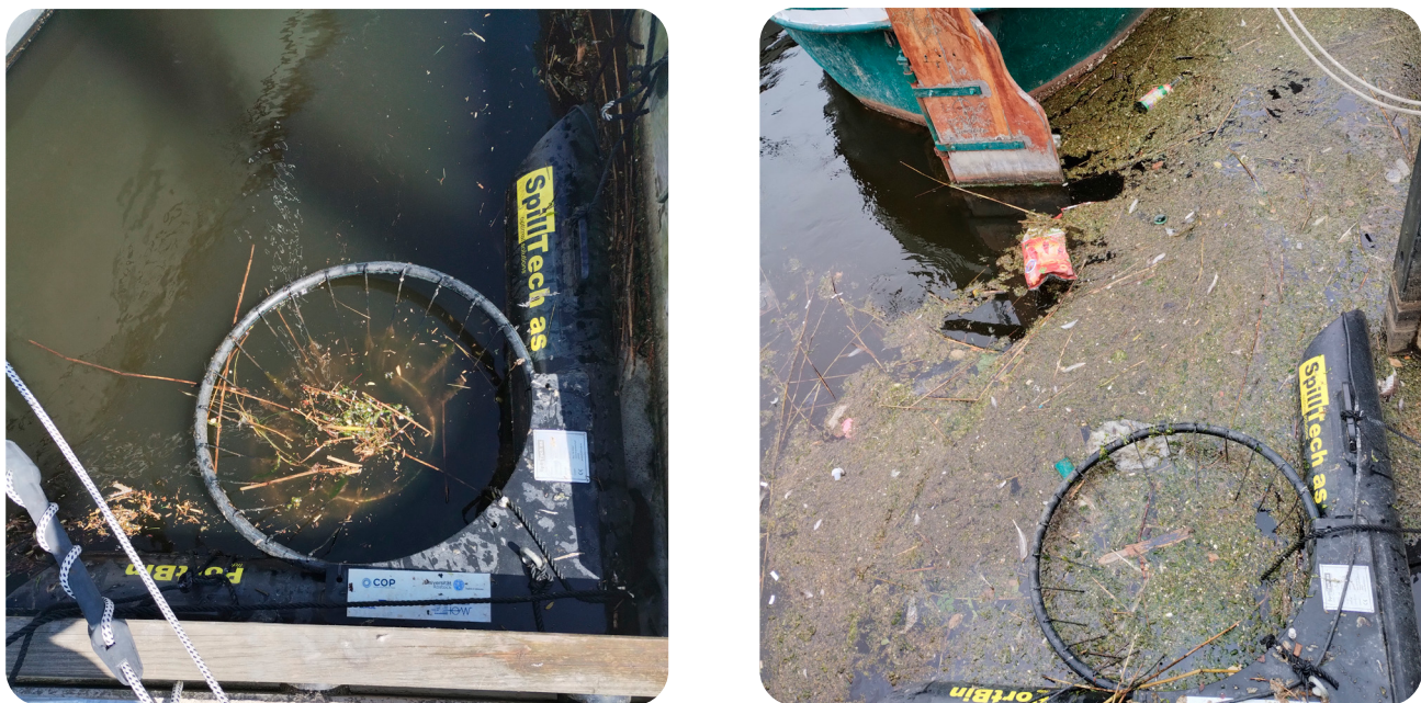
Fig.7 PortBin performance under contrasting wind conditions in the Rostock harbour basin. Under offshore wind conditions (left), only small amounts of litter and organic debris entered the PortBin. Under onshore wind conditions (right), wind pushed larger amounts of litter and organic material into the basin, quickly exceeding the PortBin’s collection capacity and leaving floating material around the device.
